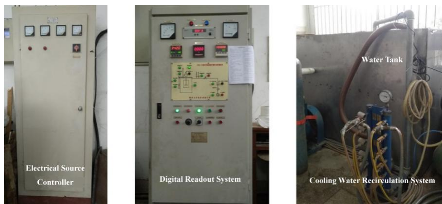
图 S3 腐蚀试验装置附属设备 Fig. S3 The auxiliary part of corrosion test equipment
